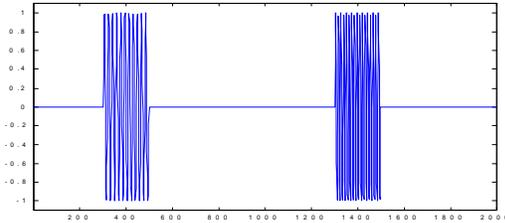
Figure 7 Tone Burst Controller Input
