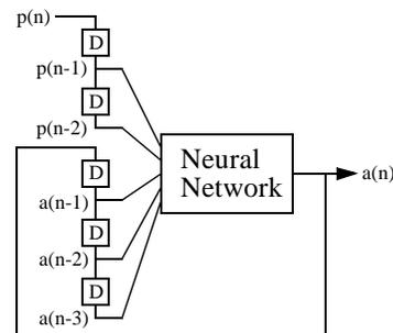
Figure 1 Time-lagged Recurrent Network
